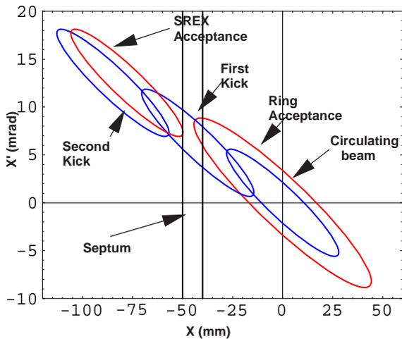
Fig: 5 The phase-space locations of the circulating beam, beam after the first kick and beam after the second kick. The ring acceptance of the ring and extraction line are also shown.
