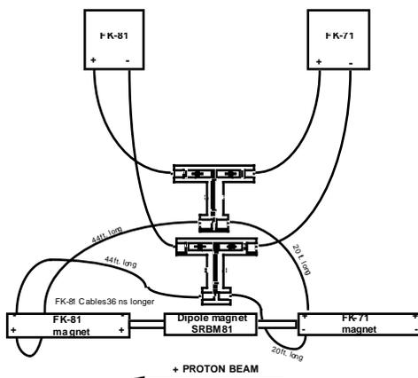
Fig: 1 Arrangement of two kickers and modulators used to deliver two pulses from PSR. In the standard mode of operation, each kicker is excited by a separate modulator.
