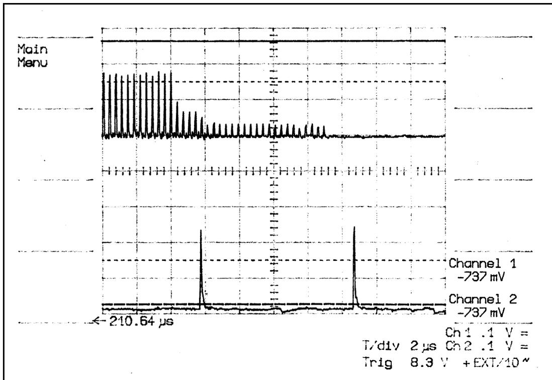
Fig: 4 The top trace shows the ring current from the wall current monitor. The bottom trace is the signal from a fast current transformer in Line-D. One time division is 2  $\mu$ s. The two modulators are fired 9  $\mu$ s apart.
