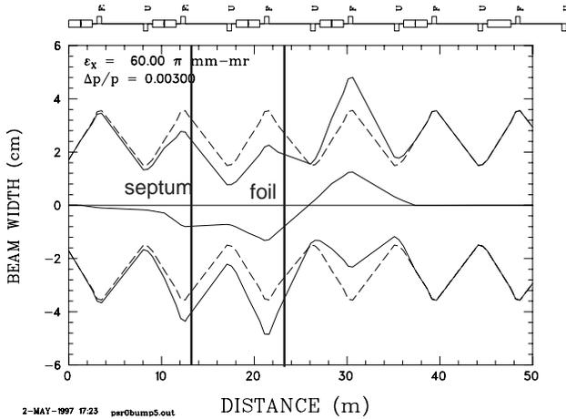
Fig: 3 The closed-orbit bump used in the two-pulse extraction experiments. Two vertical lines show the position of the septum and of the foil. The closed-orbit displacement is -8 mm at the septum, -10 mm, +3 mr at the foil.
