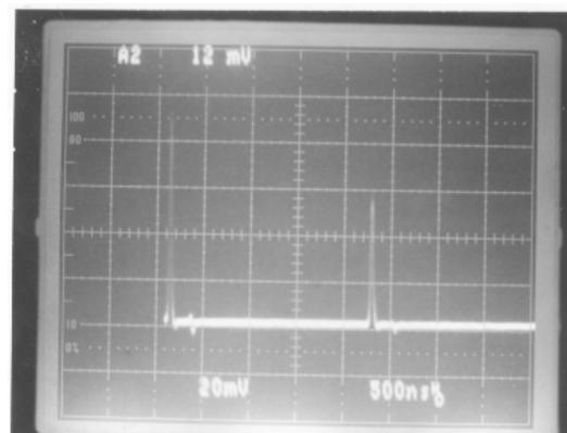
Fig: 2. Observed pulse shape in two-pulse extraction mode from PSR.
