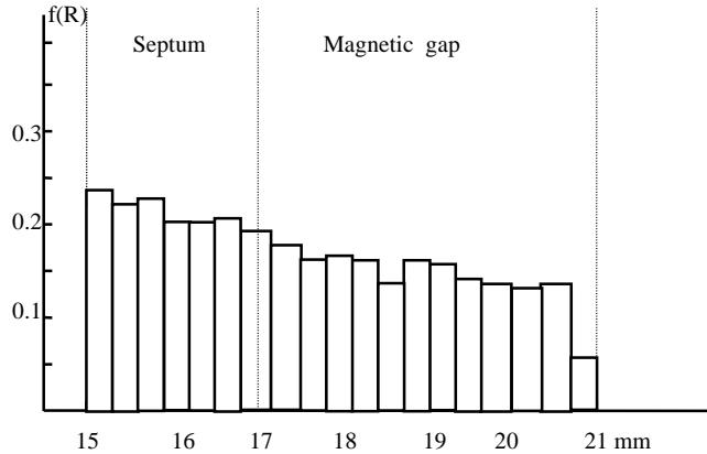
Fig.2. Conventional particles distribution in the cross section of kicker magnet at slow extraction
