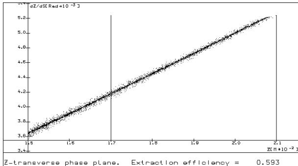
Fig.6. Beam phase portrait for ejection at conventional sextupole resonance
