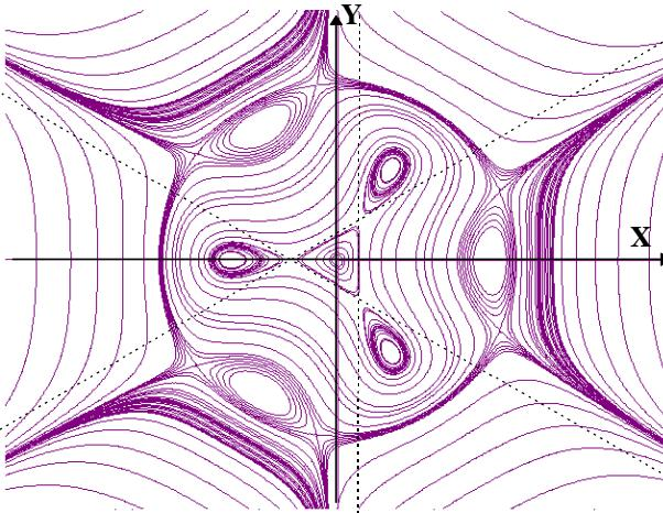
Fig.5. Phase-space trajectories near perturbed sextupole resonance
