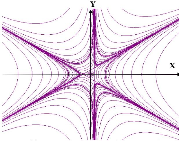
Fig.4. Phase-space trajectories near sextupole resonance
