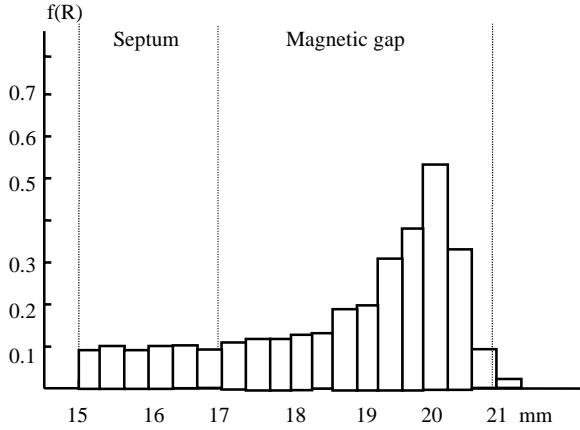
Fig.3. Optimised distribution of particles in kicker magnet cross section at decapole perturbation of sextupole resonance
