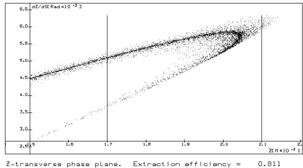
Fig.7. Beam phase portrait for ejection at perturbed sextupole resonance
