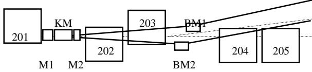
Fig.1 Schematic arrangement of beam ejection system, where K-is kicker magnet with septum, M12 - magnets for local orbit deviation, BM - bending magnets.
