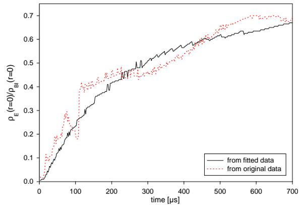
Figure: 5 Relative electron density on beam axis as a function of time.
