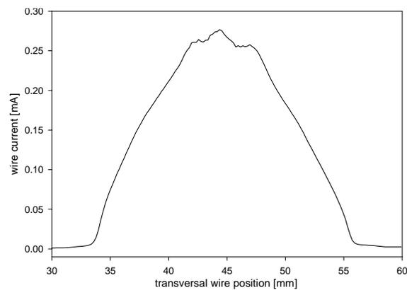
Figure: 2 Projection of beam profile measured with wire scanner.
