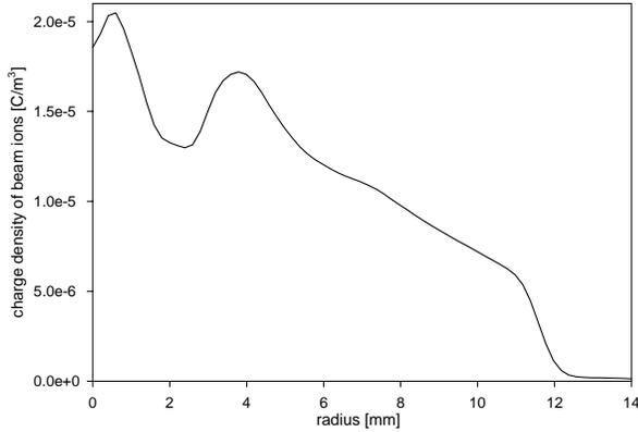
Figure: 3 Radial beam profile gained from Abel-inversion.
