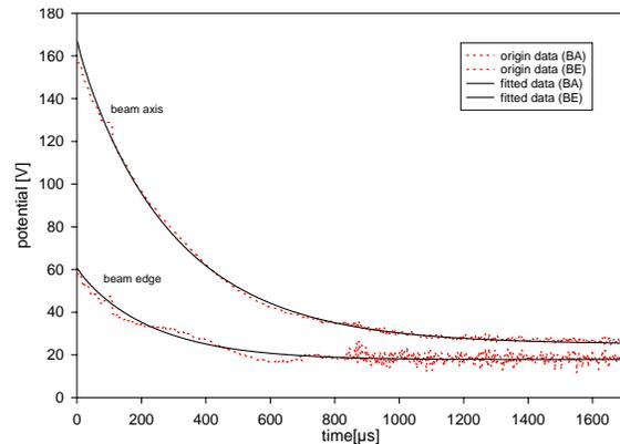
Figure: 1 Temporal development of potentials of beam axis and beam edge and analytical fit.
