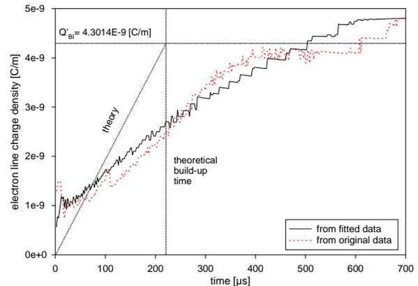
Figure: 6 Electron line charge density as a function of time.
