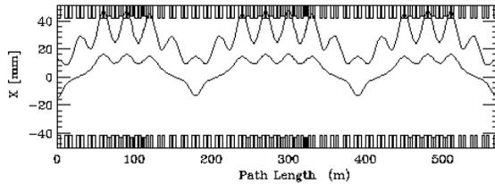
Figure 4 : Horizontal beam trajectory and envelope for a 1% systematic field (or momentum) error.
