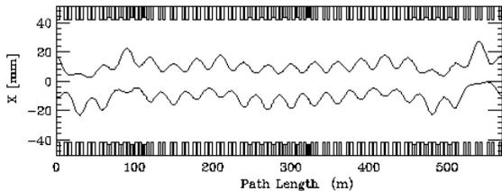
Figure 6 : Horizontal beam trajectory and envelope for the 'worst case' random 0.25% field errors.
