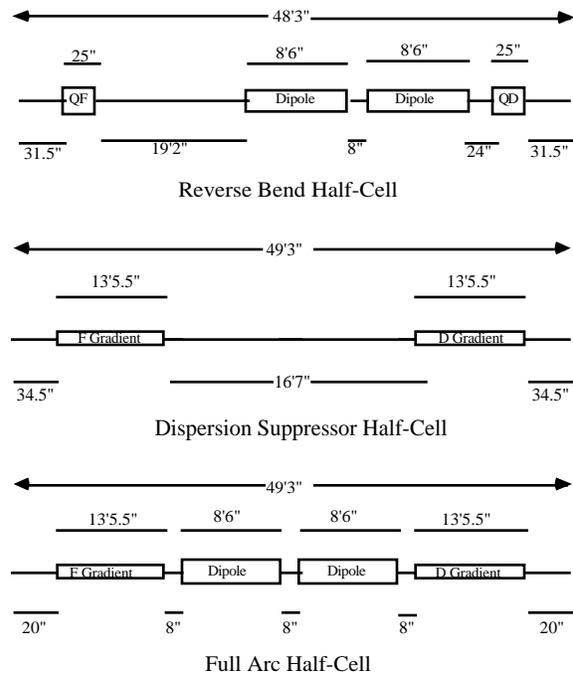
Figure 1 : Physical layout of the 3 permanent magnet cell types in the 8 GeV transfer line (not to scale).
