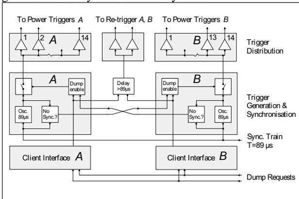
Figure 4: Client interface, trigger generation, synchronisation and distribution
