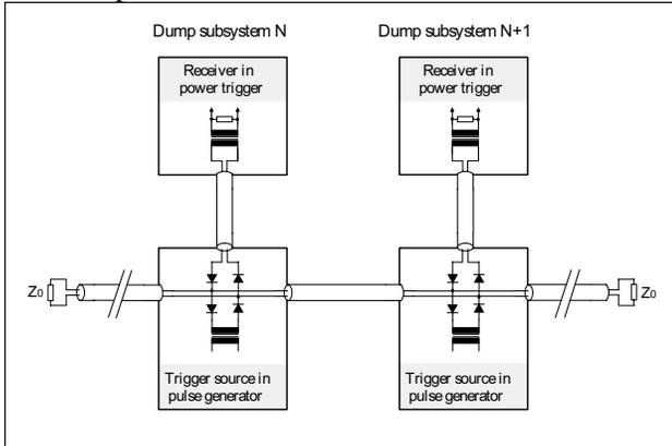
Figure 3. Principle of the re-trigger system.
