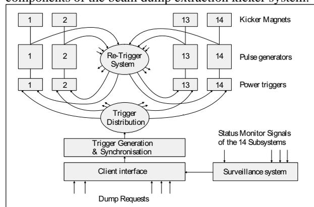
Figure 1. Functional lay-out of the dump kicker system.
