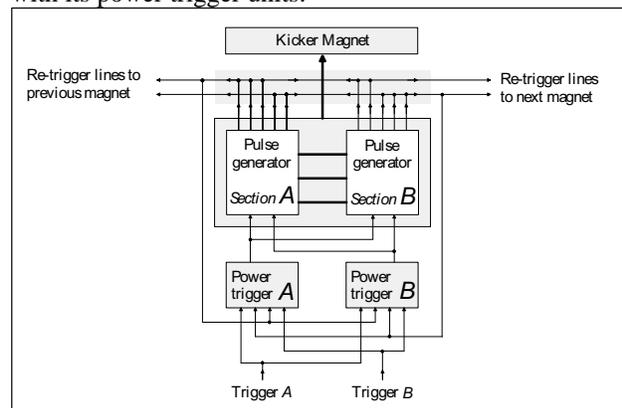
Figure 2. Block diagram of the power trigger/pulse generator/magnet chain.
