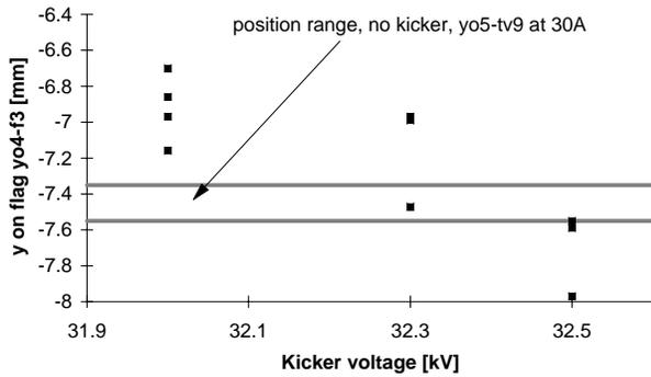
Figure 2: Measurement of the injection kicker strength. The beam was observed on a flag at the end of the sextant. The position on this flag for 3 different kicker strengths is compared with the position when the kicker was replaced by a nearby vertical corrector.
