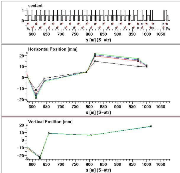
Figure 5: Injection of multiple bunches into the Sextant. Bunches are separated by 100 ms.
