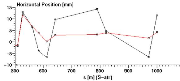
Figure 7: Correction of the horizontal orbit at injection.
