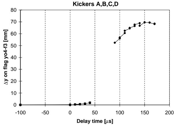
Figure 3: Rise time measurement using all four injection kickers. The beam position was observed on a flag at the end of the sextant. The left part of the curve was measured while the vertical corrector yo5-tv9 was powered at nominal strength; the right part of the curve was measured without it.
