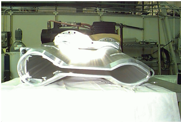
Figure 1: View of the APS storage ring Al extrusion used for vacuum chambers.
