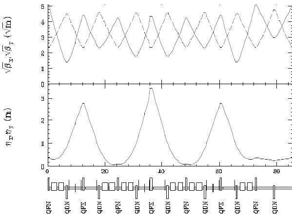
Fig. 4 Flexible momentum compaction (FMC) lattice for the 3GeV booster.
