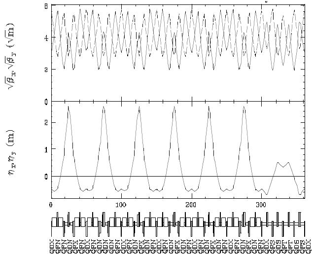
Fig. 2: Betatron oscillation amplitude and dispersion functions in the main ring. The solid line in the top is the horizontal betatron oscillation amplitude and the dashed line is the vertical one. In the bottom picture, the vertical dispersion is zero and the other curve is the horizontal one. One quarter of the ring is depicted.
