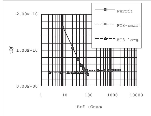
Fig.3: Characteristics of large and small FINEMET(FT3) and typical ferrite cores
