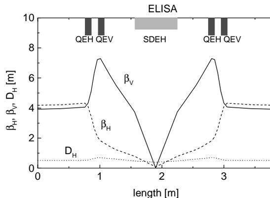
Figure 2 Lattice functions for half the circumference.
