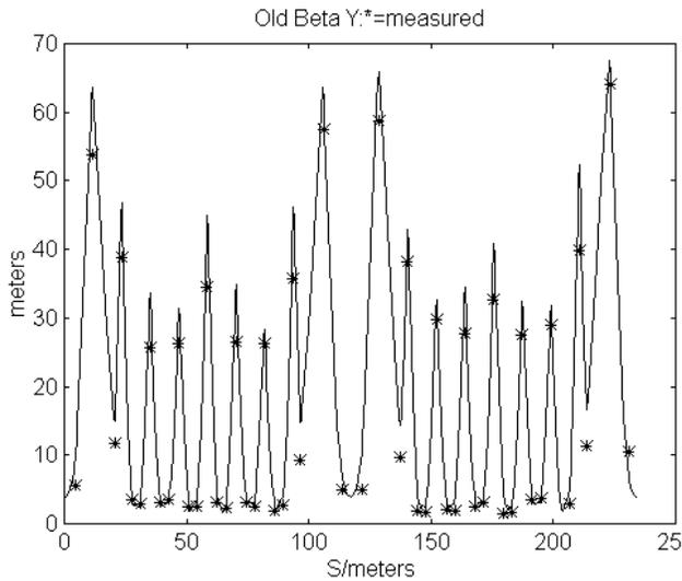
Figure 1: Vertical beta function before correction.
