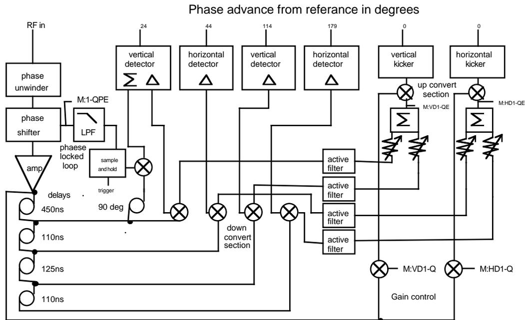
Fig 3. Block diagram of the damper system. M:1-QPE is the phase correction of the phase locked loop. M:HD1-QE and M:VD1-QE are horizontal and vertical corrections applied to the kickers. M:HD1-Q and M:VD1-Q are ramp generators which control the gain of the damper during the machine cycle.
