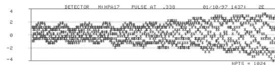
Fig 1. Turn by turn data from a BPM showing growth in horizontal betatron amplitude due to resistive wall. 1024 turns are displayed.
