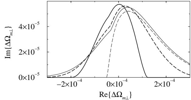
Figure 2: Stability curves for transverse tune spread, when  $v_y = 5 \times 10^{-5}$ . The thin lines are for the distribution (8), whereas the thick lines are for (9) ( $\mu = 4.5$  for the solid,  $\mu = 12.5$  for the dashed). All lines have  $v_x = -3.58 \times 10^{-5}$ , except for the thin dashed line, for which it is zero (one-dimensional).
