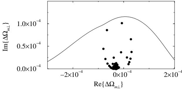
Figure 1: Example use of a stability diagram. The circles are the complex tune shifts of the transverse  $m = 1$  multi-bunch modes computed for a linear lattice. The solid line is the stability diagram. In this case, all the modes are Landau damped since they all lie below the stability curve.
