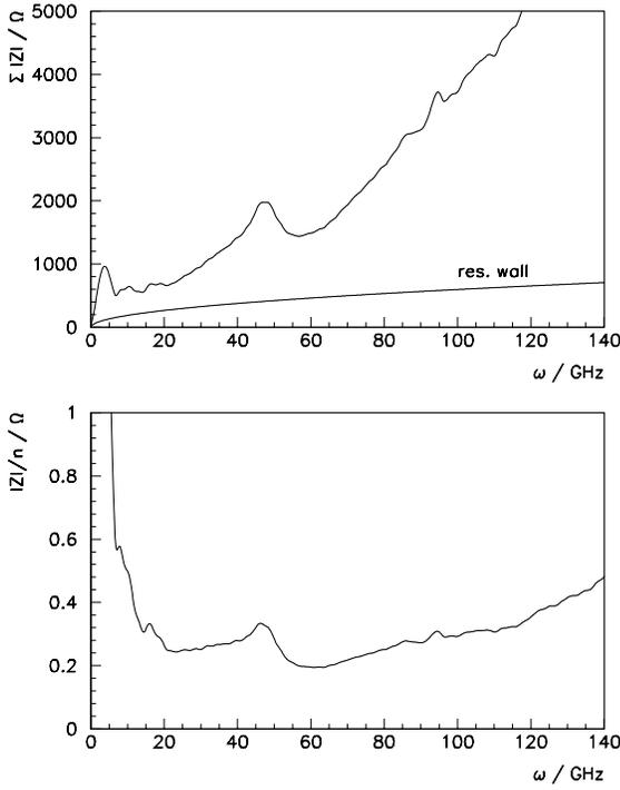
Figure 4: Summed longitudinal impedance of all components including the resistive wall impedance (top), and  $|Z/n|$  as function of frequency.
