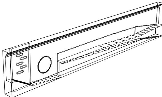
Figure 3: MAFIA 3-d model for the injection region. In this picture, the beam is injected from the right. The model includes the septum, a screen monitor and an array of pumping slots.
