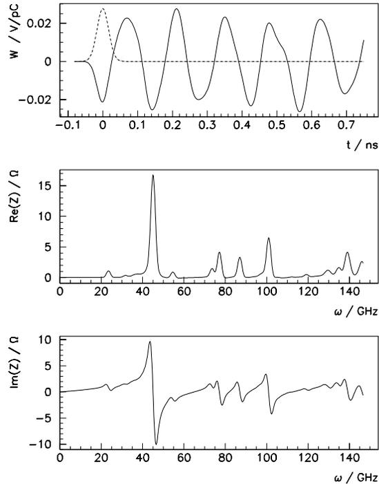
Figure 1: Wake function of a beam position monitor (top). Dividing the Fourier transform of the wake function by the bunch spectrum yields the corresponding impedance.
