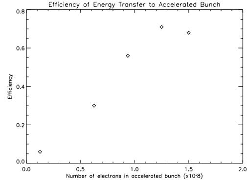
Figure 4: Acceleration efficiency  $\eta_{acc}$  as a function of beam loading.
