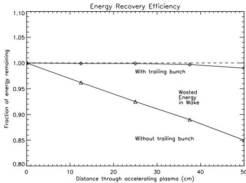
Figure 3: Fraction of energy remaining in leading half of driver bunch (diamonds) and in both halves (triangles) as a function of acceleration distance.
