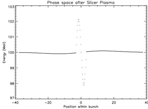
Figure 1: Electron phase space at the end of the laser-plasma scissors.
