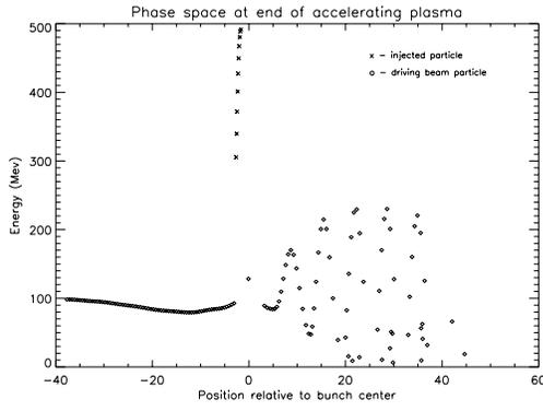
Figure 2: Electron phase space at the end of the laser-plasma scissors.
