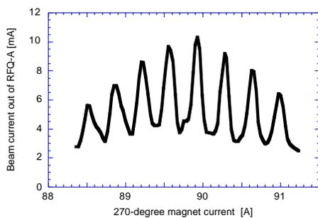
Figure 3. Current from RFQ-A as a function of 270° magnet current, with phase feedback loop off.
