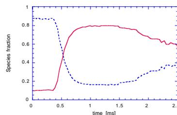
Figure 1. Yield of  $\text{He}^+$  (dashed) and  $\text{He}^{++}$  (solid) beam in the Faraday collectors as a function of stripper delay time in the prototype stripper cell for argon gas at 60 Hz.
