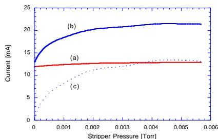
Figure 2. Current through MEBT toroids as a function of stripper pressure for nitrogen gas at 360 Hz, (a) before stripper, (b) after stripper, (c) at end of MEBT.
