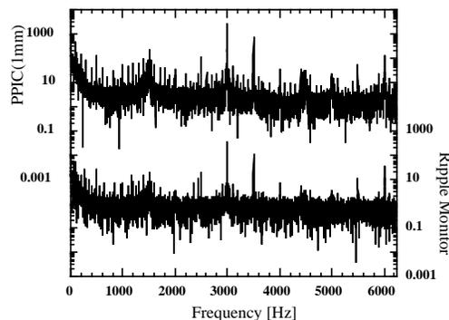
Figure 9: Frequency spectra of the signals from the PPIC(1mm) with the 759.8 Torr air (upper) and the Ripple Monitor (lower). The repetition rate of the frequency modulation of RF-KO field is 3000 Hz.
