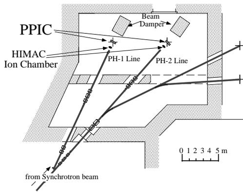
Figure 3: The plane view of the “physics and general” experimental room.
