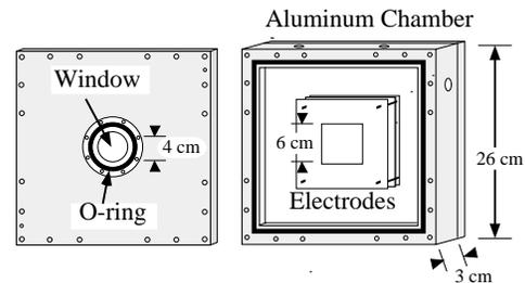
Figure 1: The PPIC. The left figure shows the front lid of the PPIC. The front and rear windows are sealed with O-rings. Three electrodes are mounted in the aluminum chamber.
