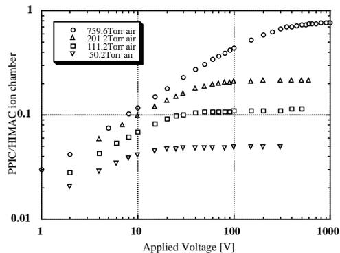
Figure 6: The plateau curve of PPIC(3mm gap distance) with air. The beams are  $1.3 \times 10^9$  pps  $C^{6+}$  (290 mev/u). The ordinate is the ratio between the output charge from the PPIC and the HIMAC ion chamber.
