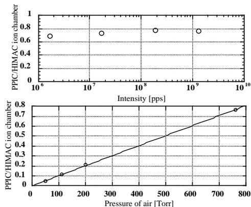
Figure 7: The PPIC signal dependence on the intensity (upper) and the pressure of the counter gas (lower).
