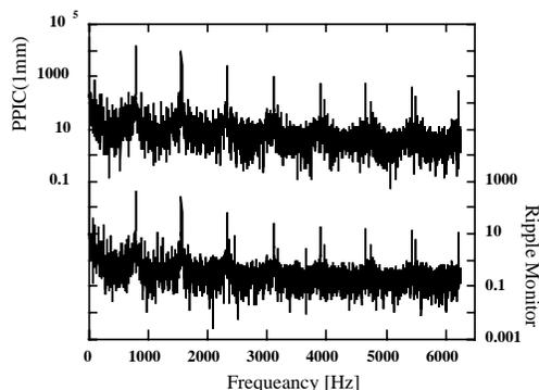
Figure 8: Frequency spectra of the signals from the PPIC(1mm) with the 759.8 Torr air (upper) and the Ripple Monitor (lower). The repetition rate of the frequency modulation of RF-KO field is 777 Hz as usually use for therapy.
