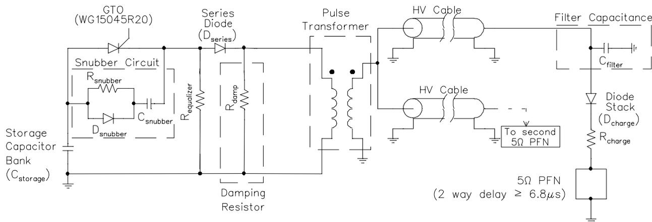
Figure 1. Schematic of Resonant Charging Supply
