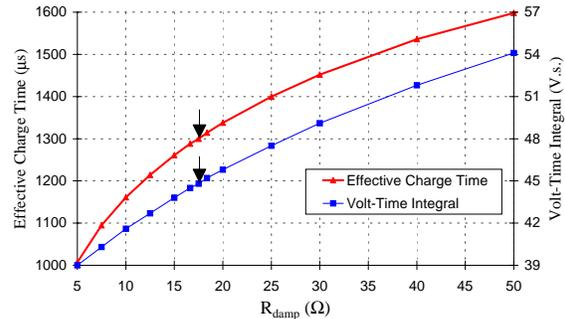
**Figure 3. ECT and VTI as a function of the value of the damping resistor**
