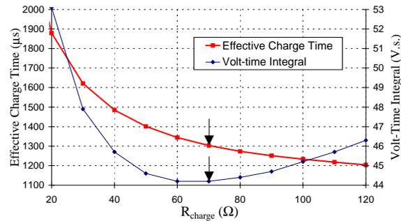
**Figure 6. ECT and VTI versus the value of the charging resistor ( $C_{\text{filter}} \times R_{\text{charge}} = 360$  ns)**
