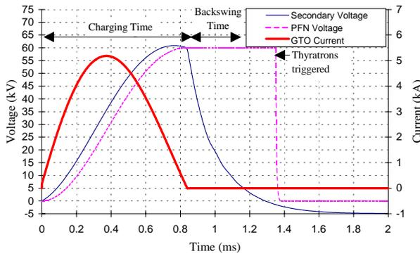
**Figure 2. Typical secondary voltage, PFN voltage and GTO current waveforms**
