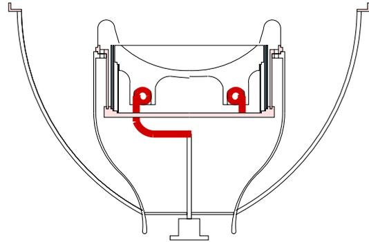
Figure 1: Cut-away section of dispenser cathode assembly in high voltage ceramic bushing
