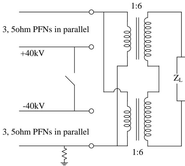
Figure 1: Schematic of pulse transformer.
