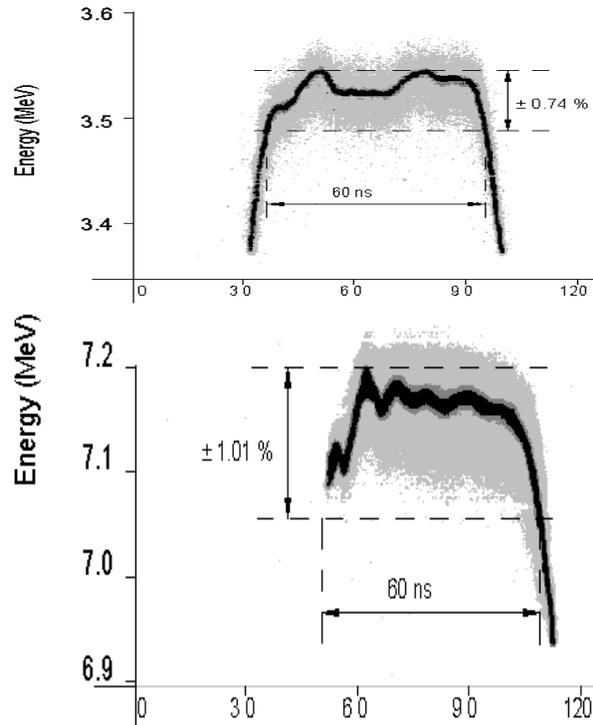
Figure 2: Beam energy spectrums at injector output (3.55 MeV) and 16 cells accelerator output (7.2 MeV).
