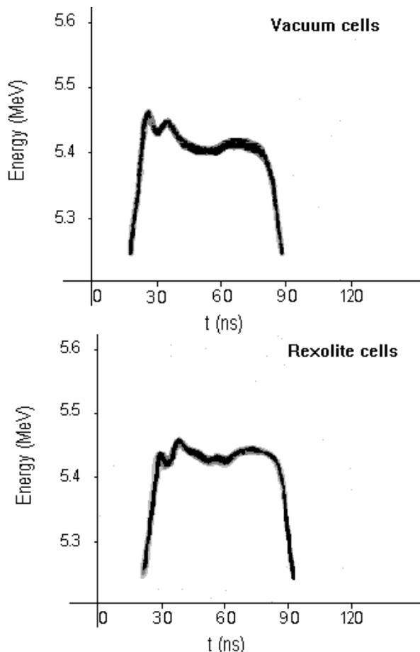
Figure 3: Energy spectrums obtained after acceleration with Rexolite or vacuum cells.
