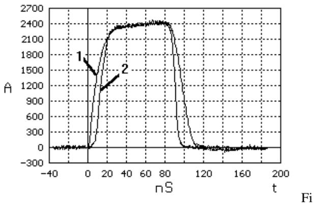
Figure 1: Beam profile at injector output (1) and accelerator output (2).
