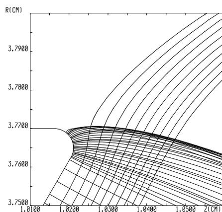
Fig. 3. Some equipotentials and trajectories near the cathode edge.
