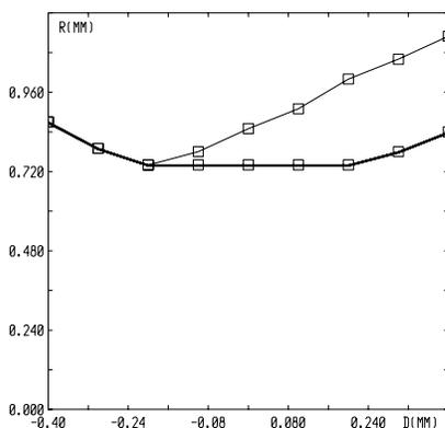
Fig. 6 The beam radius in the magnetic system versus the cathode position for optimal negative voltage (lower curve) and with zero voltage (upper curve).
