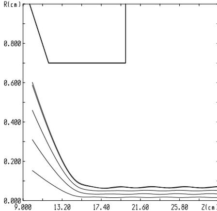
Fig. 5. The beam envelopes containing 6%, 25%, 56%, 95%, 100% of total current, respectively.
