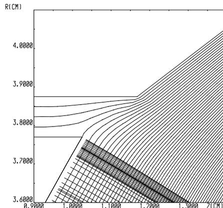
Fig. 2. Equipotentials and trajectories near a gap between the cathode and the focus electrode.
