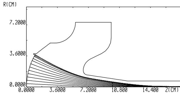
Fig. 1. The gun layout and electron trajectories
