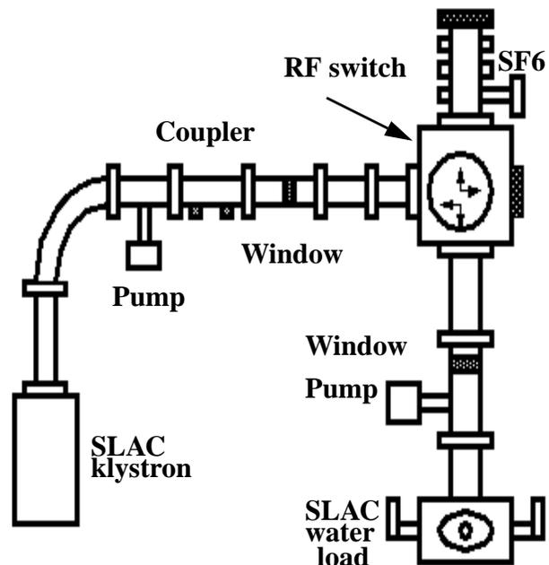
Figure 1: Schematic layout of the rf pressurized waveguide switch test.
