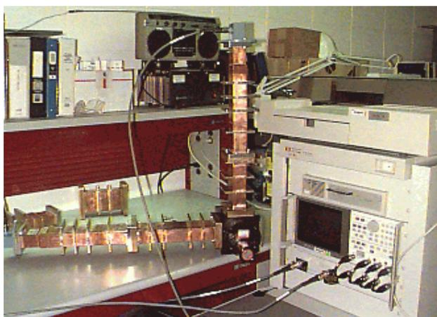
Figure 6: Network analyzer measurements of the WR-340 switch and tapered transitions.
