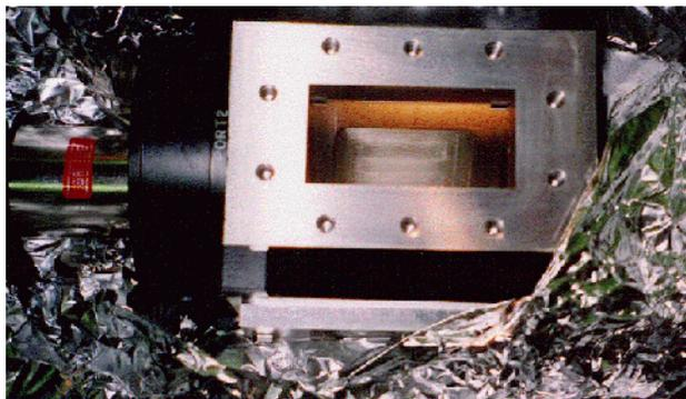
Figure 3: Vendor 2's WR-340 waveguide switch.
