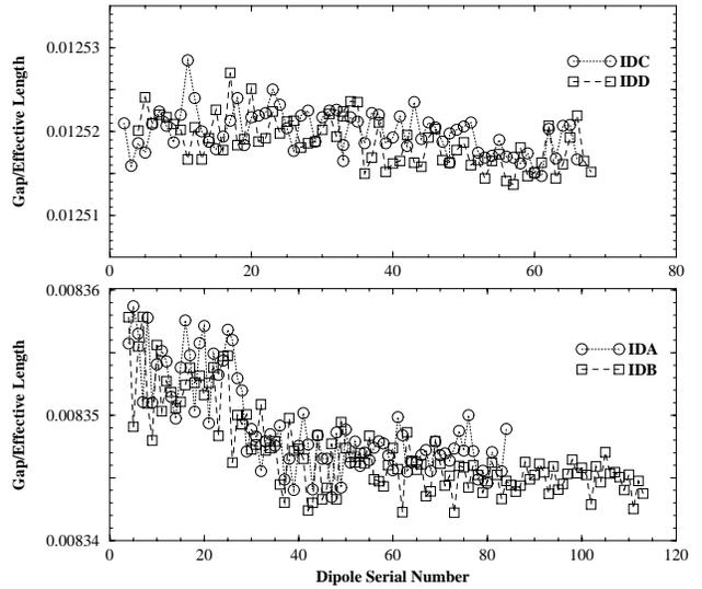
Figure 5:  $g/L_{eff}$  for 6 m (below) and 4 m (above) dipoles vs. production serial number. The apparent change after IDA028 and IDB025 and the subsequent improved uniformity is believed to be due to several improvements in the half core manufacture and magnet assembly procedures. The relative change in  $g/L_{eff}$  is  $\approx 10^{-3}$ .
