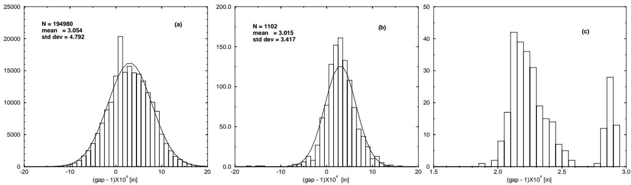
Figure 3: Measured gap (half) height distributions. (a) All measured laminations. (b) Averaged over slit coils. (c) Average gaps for half core recipes.
