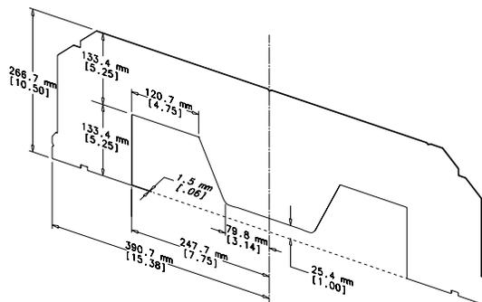
Figure 2: Main Injector dipole lamination.
