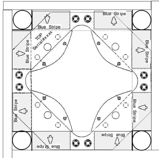
Figure 1 Magnet Cross Section, ferrite bricks are dotted.
