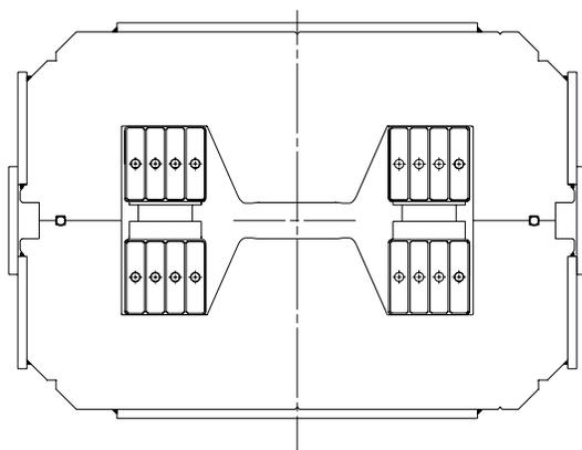
Figure 2. Cross-section of machined dipole. For scale, the lamination is 78.1 cm x 26.7 cm.
