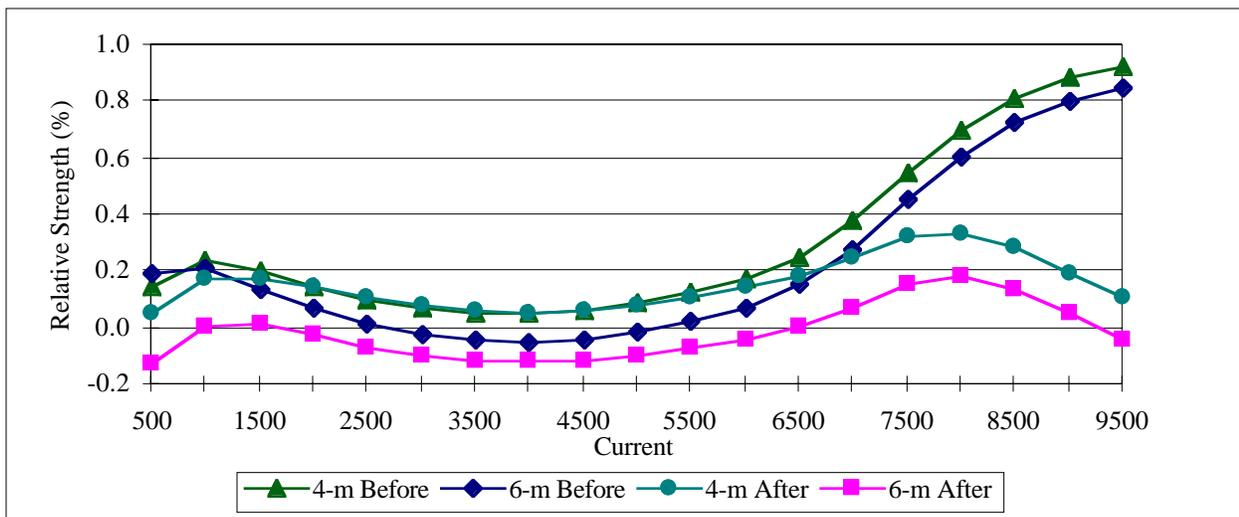
Figure 1. Dipoles strengths, relative to production magnets, for the pre-production magnets before and after machining.
