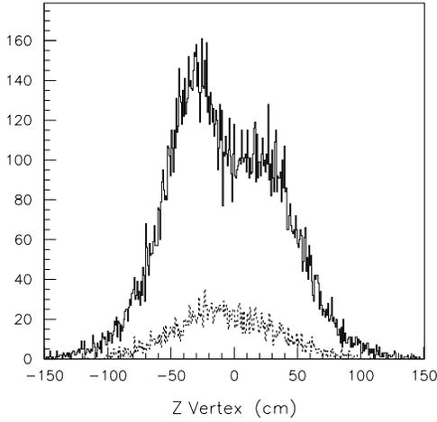
Figure 1: Longitudinal Luminosity Profile for beams separated horizontally by  $100 \mu\text{m}$ . Solid lines are Single Interaction, and dashed lines are Multiple Interaction events.
