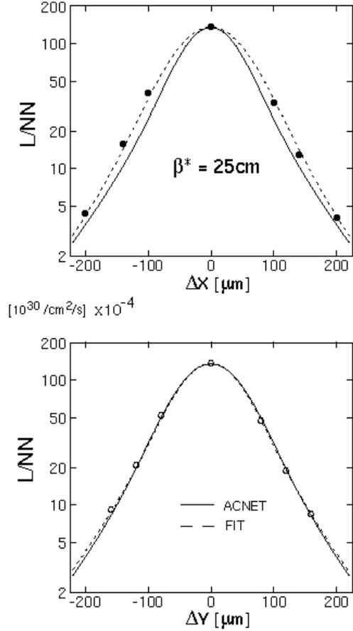
Figure 2:  $\mathcal{L}/(N_p N_a)$  versus separation for X and Y scans; the overlaid model calculations use accelerator- (solid line) or fit separated beam- (dashed line) parameters and have been scaled to agree at zero separation.
