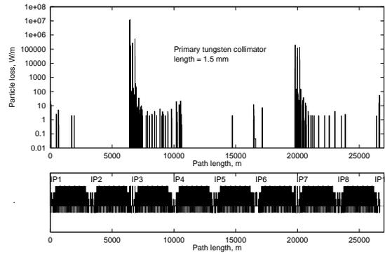
Figure 4: Beam loss distribution in the LHC lattice at injection with a 1.5 mm tungsten primary collimator.
