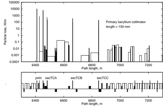
Figure 1: Beam loss distribution in the IP3 beam collimation region at collisions for 150 mm beryllium primary collimator.
