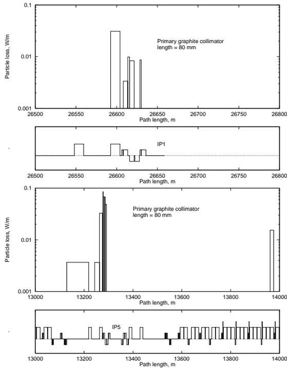
Figure 3: Beam loss distribution in IP1 (top) and IP5 (bottom) at collisions with simultaneous amplitude and momentum cleaning with a 80 mm graphite primary collimators.
