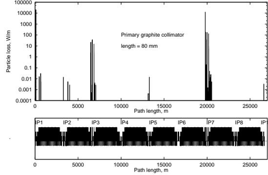
Figure 2: Beam loss distribution in the LHC lattice at momentum cleaning for a 80 mm graphite primary collimator in IP7.
