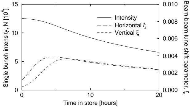
Figure 6: Long range tune shift evolution, per IR.
