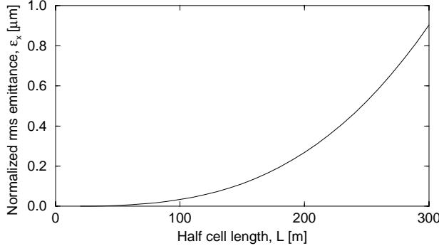
Figure 1: Equilibrium emittance versus half cell length
