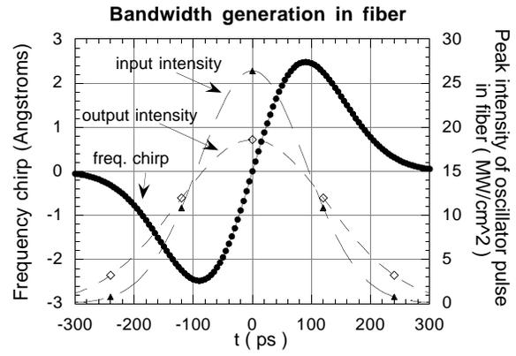
Figure 3: Intensity of input and output laser pulse and chirping introduced on the output pulse due to SPM and GVD from the fiber.
