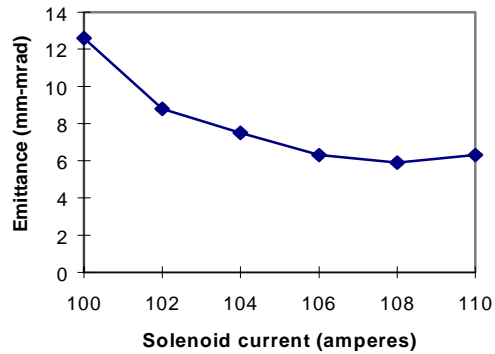
Figure: 3 Normalized total vertical emittance measured as a function of solenoid current.
