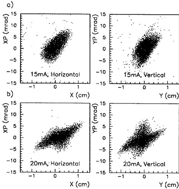
Figure 5: Measured phase-space distributions at TDEM1 for (a) 15 mA peak current beam and (b) for 20 mA current peak beam.
