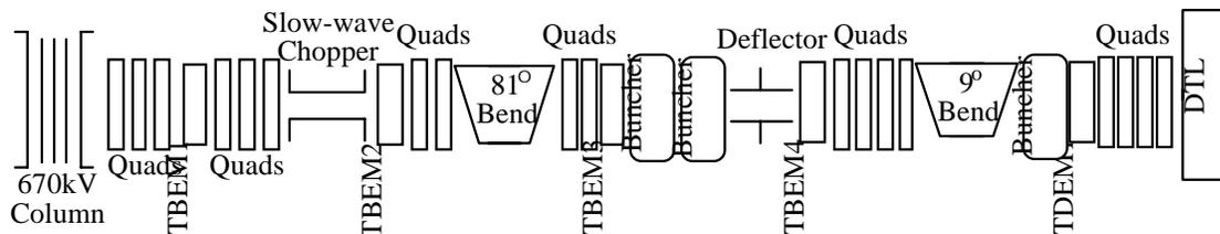
Figure 2: Schematic of the 670 kV column and 750 keV LEBT
