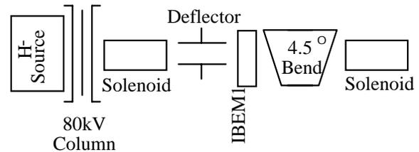
Figure 1: Schematic of the  $H^-$  source, 80 kV column and LEBT
