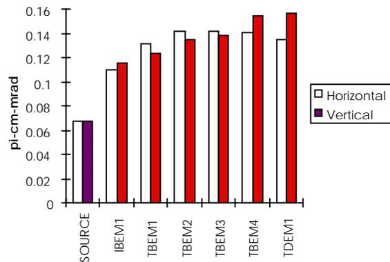
Figure 3: Total normalized emittance for 15 mA beam in LEBT.
