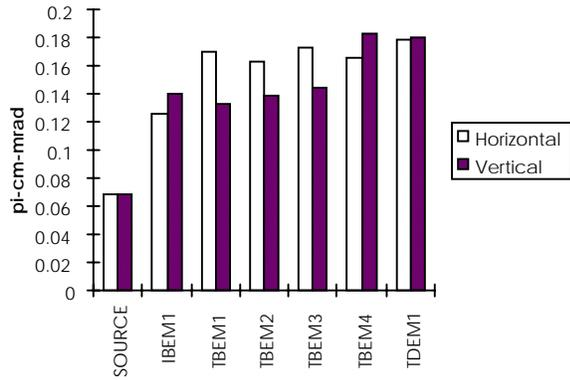
Figure 4: Total normalized emittance for 20 mA beam in LEBT.
