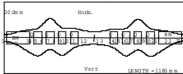
Fig.3 Beam envelope transportation along the trap, from the entrance of the first bending magnet to the entrance of the electron collector. The central region is the trapping region.
