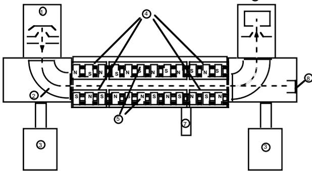
Fig.1 Operation scheme of TIS: 1) electron gun, 2) bending magnet, 3) vacuum pump, 4) static potential electrodes  $U_0$  for longitudinal ion trapping, 5) rf quadrupole electrodes with inside the focusing magnetic quadrupoles, 6) electron collector, 7) gas-inlet, 8) ion collector.
