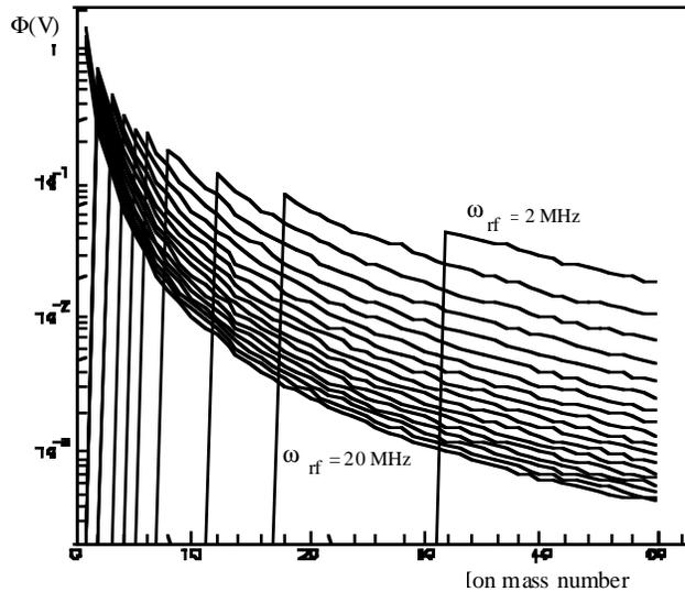
Fig.2 Potential well depth vs ion mass numbers at 1 cm from the axis for different rf frequency.
