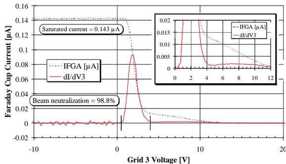
Figure 3. The FGA Faraday cup current and its derivative with respect to grid 3 voltage are plotted vs.  $V_3$ .
