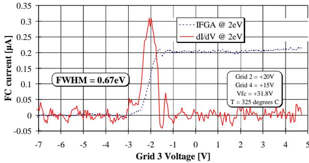
Fig. 2. Electron gun calibration of the FGA.
