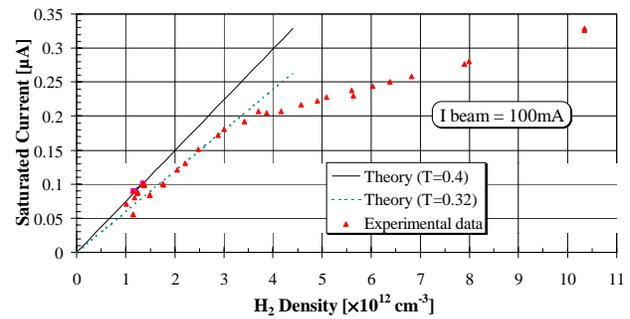
Fig. 4. Comparison of the measured and calculated FGA saturated currents.
