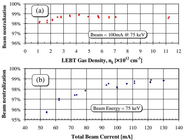
Figure 5. Plot of  $f$  vs. (a) the  $\text{H}_2$  gas density in beam transport, and (b) total beam current.
