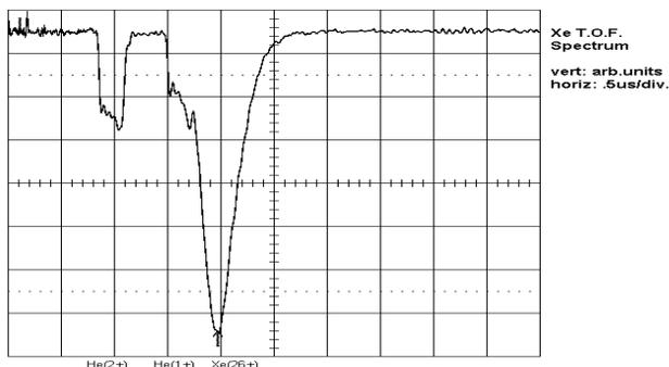
Figure 2 Xenon time-of-flight spectrum, with a peak at 26+.
