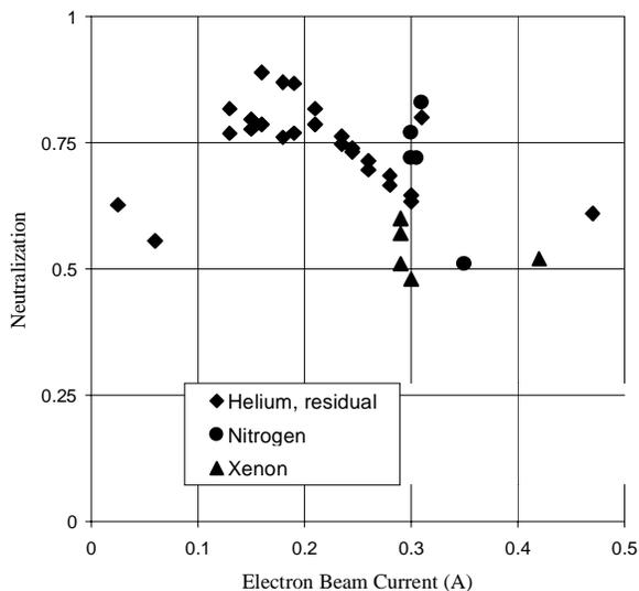
Figure 1 Neutralization vs. electron beam current, taken under various conditions.
