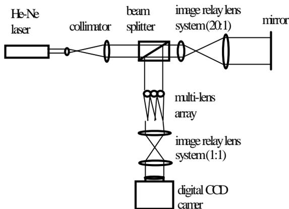
Fig. 2 the system of the Shack-Hartmann wavefront sensor
