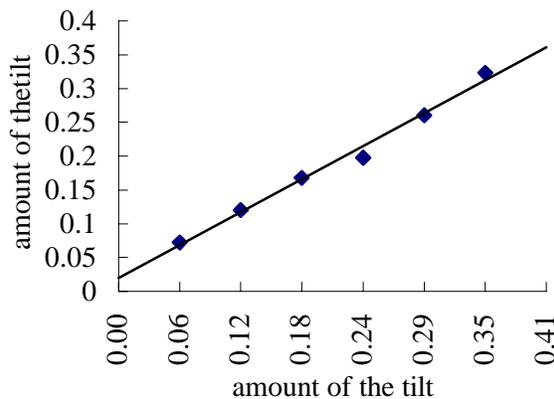
Fig. 4 Angular response of the Shack-Hartmann wavefront sensor
