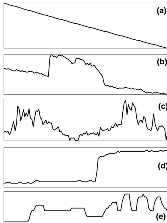
Fig. 1 Typical system performance over a two-hour period (horizontal axis) that includes a 35-minute beam noise. **a** beam current (96.2 to 90.6 mA), **b** Beamline 10 sum (0.13V span, 1.47V min.), **c** cavity temperature (between 48.4 to 48.9 deg C), **e** tuner #1 position (0.34 mm span), **f** tuner #5 position (0.11 mm span). All scales are linear.
