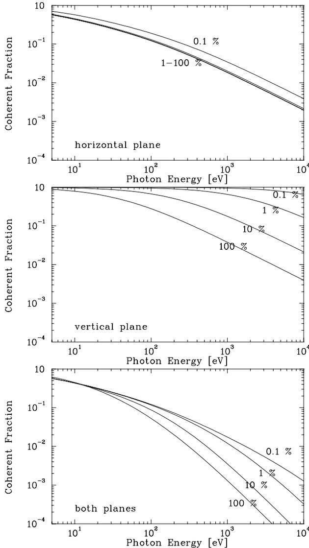
Figure 2: Coherent fraction of undulator radiation for (a) the horizontal plane, (b) the vertical plane and (c) the combined effect.
