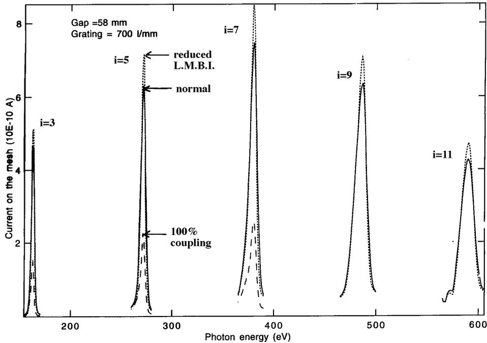
Figure 1: Line spectra taken on the ID\_3, VUV beamline as a function of the different methods to increase the beam lifetime. Spectra shown refer to reduced longitudinal multibunch excitation, normal operating conditions (x2 increase in energy spread) and 100 % coupling.
