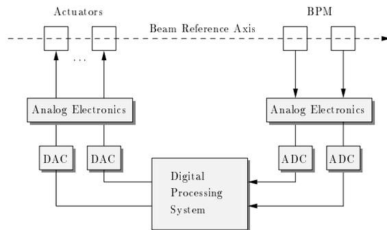
Figure 1: Schematic diagram of digital feedback systems
