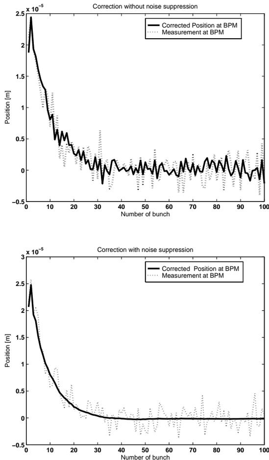
Figure 2: Simulation plots of fast feedback (BDS): Position and measurement 1) without and 2) with noise suppression. For scaling reasons, the offset of the pilot bunch ( $45 \mu\text{m}$ ) is not shown.
