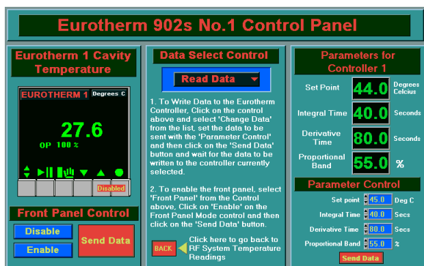
Figure 3: The LabVIEW® cavity body temperature control application for a Eurotherm 902s Controller.
