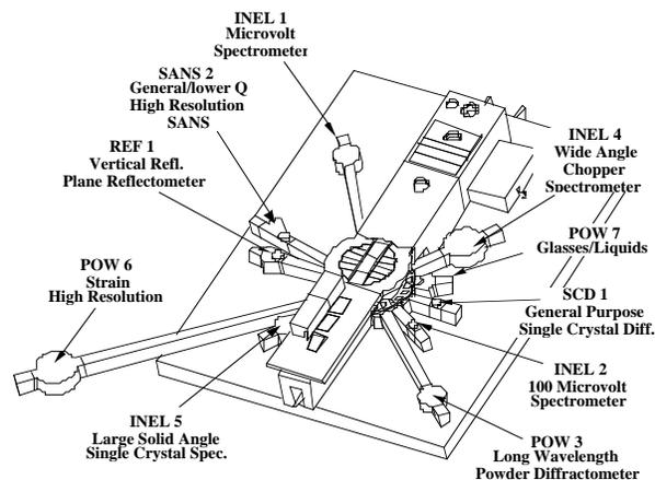
Fig. 3. Layout of experimental hall showing neutron beam lines and initial instrument set.
