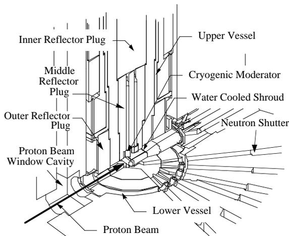
Fig. 2. Cross-sectional view of target station.
