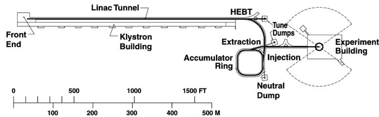
**Fig. 1. Schematic representation of the accelerator system layout and experiment building for the first 1-MW phase of NSNS.**
