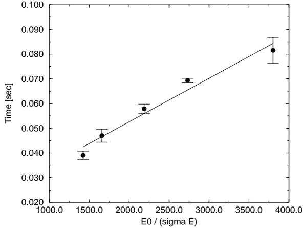
Figure 5: Peak separation of double-peaked echoes,  $\Delta t_{peak}$ , versus the inverse of  $\frac{\sigma_E}{E_0}$ , the energy spread of the beam. The value of the slope from the linear fit is 1.76E-5. The beam parameters were  $I_0 = 147$  mA,  $\eta = .023$ ,  $\beta^2 = .988$ ,  $h_{echo} = 1$ , and  $f_{rev} = 629$  kHz.
