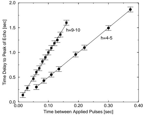
Figure 2: Measured echo delay time as a function of separation of the drive pulses. Upper curve: 1<sup>st</sup> pulse at  $h = 9$ , 2<sup>nd</sup> pulse at  $h = 10$ , giving expected time dependence  $t_{echo} = [10/(10 - 9)]\Delta t = 10\Delta t$ . Lower curve: 1<sup>st</sup> pulse at  $h = 4$ , 2<sup>nd</sup> pulse at  $h = 5$ , giving  $t_{echo} = [5/(5 - 4)]\Delta t = 5\Delta t$ .
