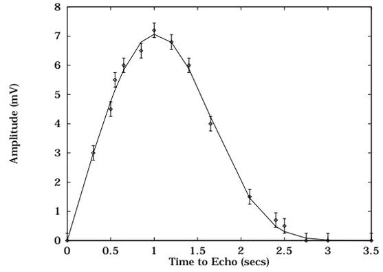
Figure 3: Peak echo response as a function of the time to echo following the initial pulse. The solid line represents a theoretical fit corresponding to a collision rate  $\nu = (3.0 \pm 0.8) \times 10^{-4}$  Hz.
