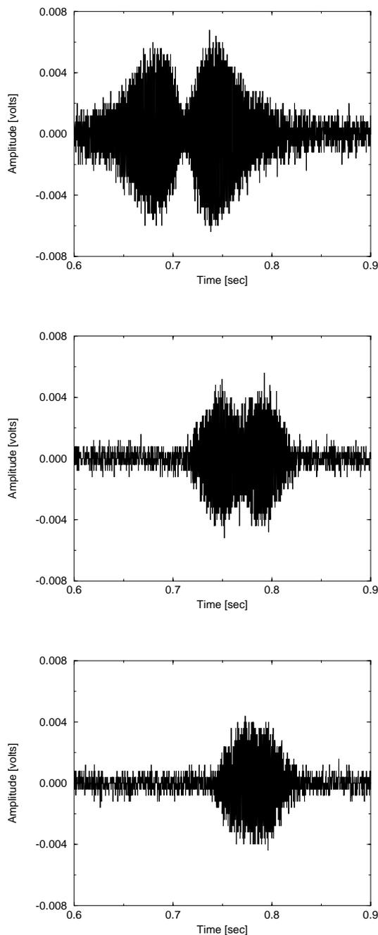
Figure 7: Three longitudinal beam echoes occurring in beams with different energy widths. The beam energy sigmas ( $\sigma_\epsilon$ ) were from top to bottom, 4.0, 6.1, and 8.0 MeVc. The energy spread was controlled with longitudinal stochastic cooling systems, all other beam conditions were the same. The beam intensity was 147 mA. Echoes which occurred at nearly the same time relative to the driving pulses were chosen for comparison.
