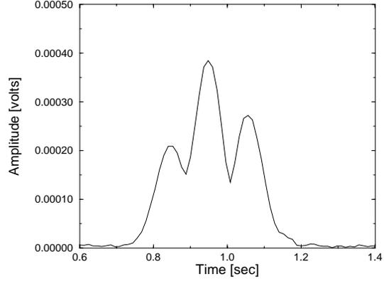
Figure 6: Beam echo from a non-Gaussian beam.
