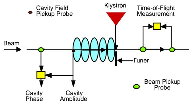
Figure 2. A schematic of the setup for calibrating phase and amplitude of SC cavities
