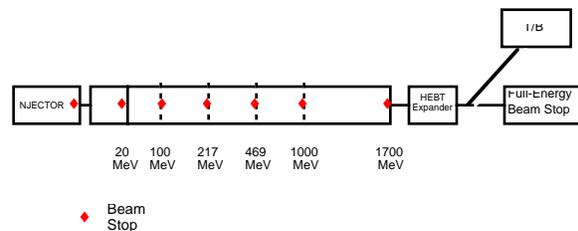
Figure 1. Schematics of APT Linac for Commissioning
