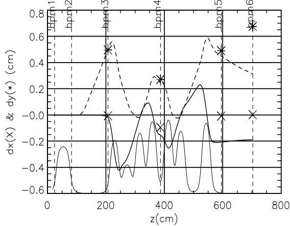
Fig.6 Centroid trajectories with bpd at edge
