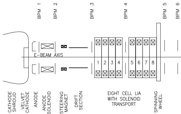
Fig.1 Layout of the ITS steering experiment
