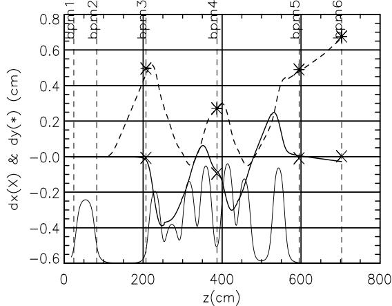
Fig.5 Centroid trajectories  $dx$  and  $dy$  through ITS
