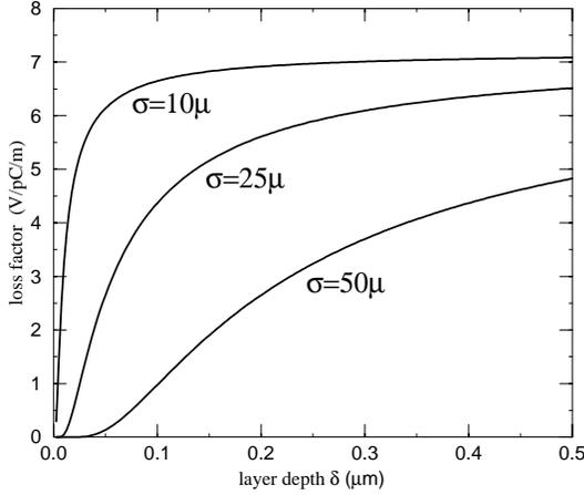
Figure 2: Loss factor (in V/pC/m) vs. layer thickness for different bunchlengths  $\sigma= 10, 25$  and  $50 \mu$
