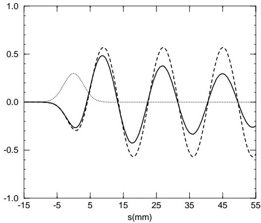
Figure 4: Normalized wake potentials ( $\sigma=3$  mm) in a "real" tube, filled with randomly spaced protusions (solid line) and filled with dielectric material (dashed line).
