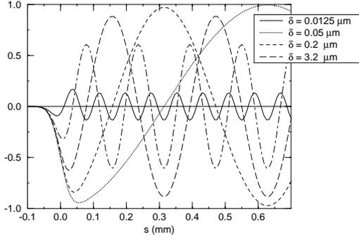
Figure 1: Wake potentials of a  $25 \mu$  bunch in the tube of the radius  $a=50$  mm for different thickness of dielectric layer  $\delta=0.0125, 0.05, 0.2, 0.8$  and  $3.2 \mu$
