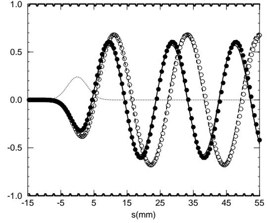
Figure 3: Normalized wake potentials ( $\sigma=3$  mm) in slightly corrugated tube (dark lines) for periods 1.25 and 4.5 mm (solid lines) and 2.5 mm (dashed line) and in tubes covered with ceramic layer (same thickness as radial size of protuberances) of dielectric constant 2 (empty circles) and 1.6 (solid circles).
