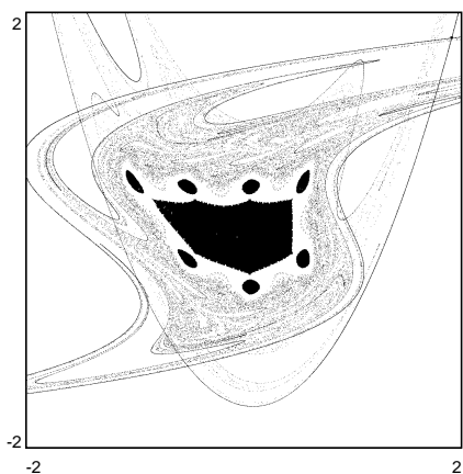
Figure 1: Stability domain (black area) and the invariant manifolds emanating from the unstable fixed point of period one of \mathbf{h}_6 .
