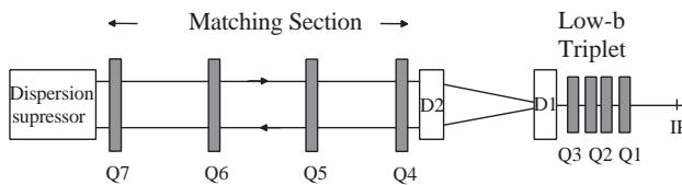
Figure 3: Lay-out of the experimental insertions
