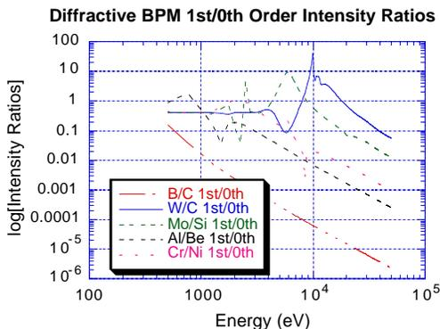
**Figure 3.** Modeled 1st/0th order diffracted intensity ratios.
