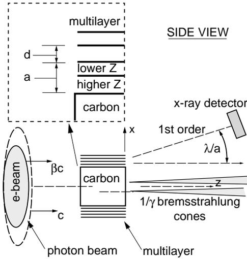
Figure 1. Diffractive wire-BPM structure.
