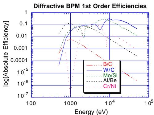
**Figure 2.** Modeled absolute BPM x-ray diffraction efficiencies.
