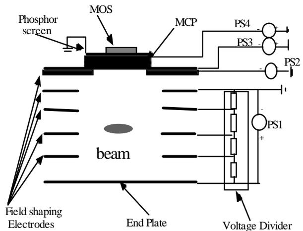
Fig.1 Operation scheme of RG-BPM.
