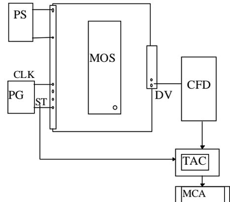
Fig.3 Block diagram of the experimental set-up for the counting mode operation of the RG-BPM: (PS) Power Supply, (PG) Pulse Generator, (CFD) Constant Fraction Discriminator, (TAC) Time to Amplitude Converter, (MCA), Multi-Channel Analyser.
