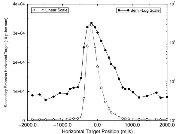
Figure 3: Secondary Emission from target for Horz. Scan
