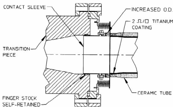
Figure 2 - Ceramic Tube End Joint Design
